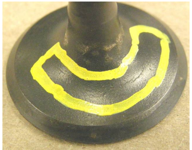
Figure 26: Cracked Valves from E15 Verado 1B812776, Bottom Valve in Cyl. 3 Left, and Top Valve in Cyl. 6 Right
